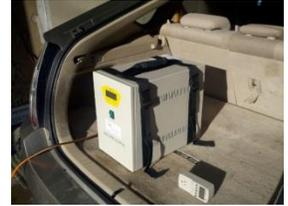
The Plug-Out and Prius combo make a phenomenal generator. Think about it. The Prius is already a great DC generator with motor and generator keeping the hybrid battery full. The Plug-Out Inverter adds high quality, pure sine wave, AC power output from the hybrid's battery. This combination yields many advantages over mechanical generators:
